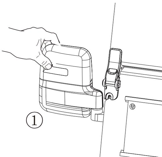
1.PUSH THE TIP OF THE REAR VIEW MIRROR INWARDS(PIC ①).
