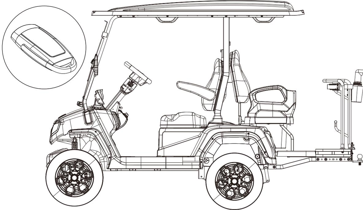
KEEP THE KEY FOB INSIDE / CLOSE TO THE VEHICLE ( MAXIMUM DETECTION DISTANCE 3.3 FEET )
