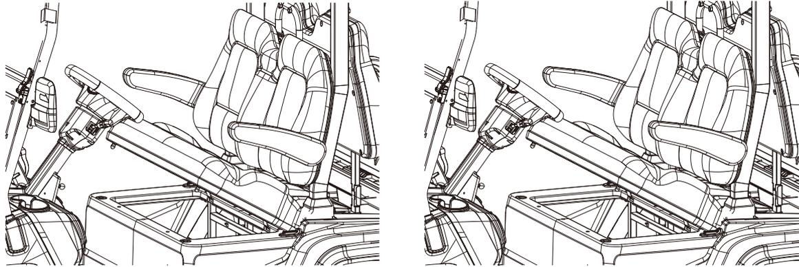
1. LIFT THE SEAT FROM THE FRONT SO THAT THE BALL AT THE BOTTOM OF THE SEAT SEPARATES FROM THE SOCKET ON THE BARREL.
