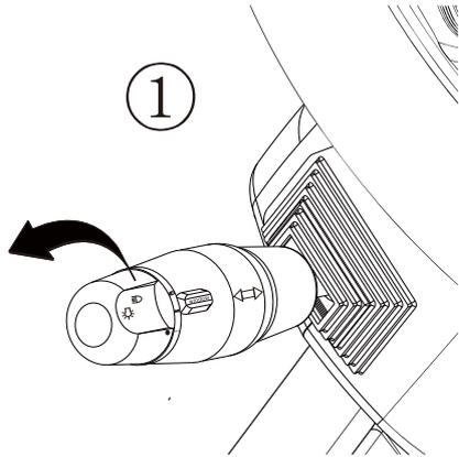
1. ROTATE THE LIGHT CONTROL KNOB TO ENABLE HEAD LIGHTS (LOW BEAM)
