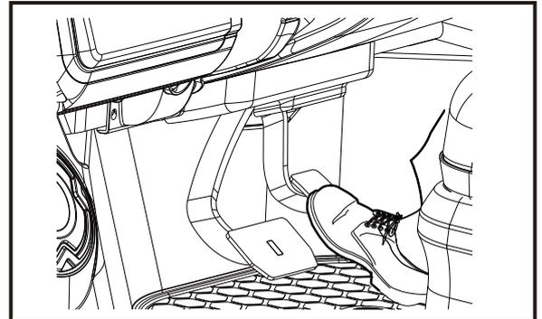
Check the brake pedal , when stepped it should be flexible and feels firm . And it returns to its original position with flexibility when released.
