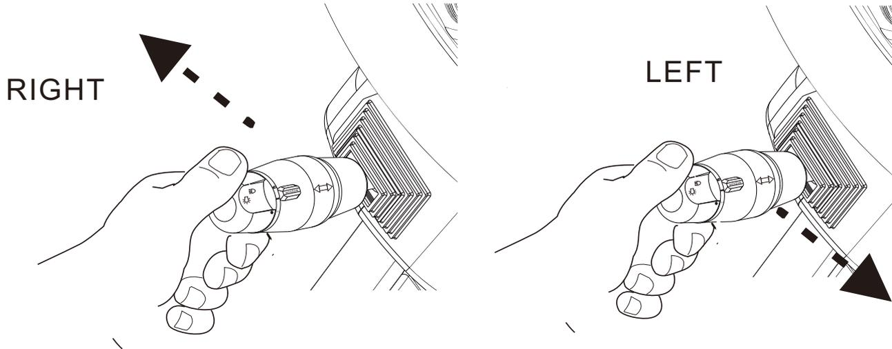
PUSH & PULL THE CONTROL STALK FORWARDS OR BACKWARDS TO ENABLE LEFT TURN SIGNALS OR RIGHT TURN SIGNALS .
