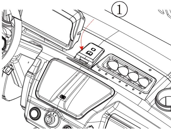
1.REMOVE THE BRAKE OIL POT COVER ON THE DASHBOARD TO GET ACCESS TO THE OIL TANK.
