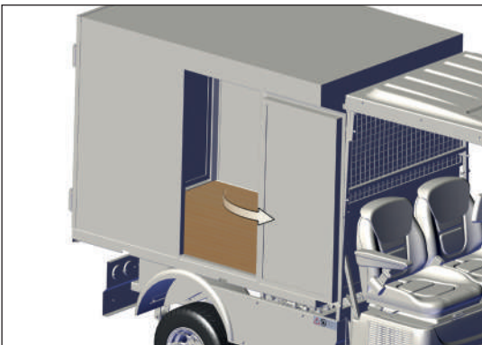
Figure 11-10 Opening the closed cargo box side cover
