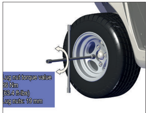
Figure 12-14 Removing the lug nuts
